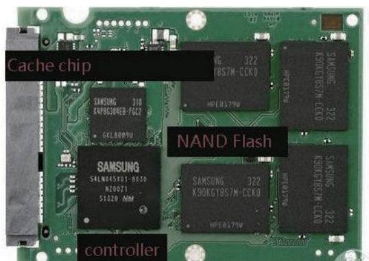
Figure 6 SSD Internals (Samsung 840EVO) [10]
